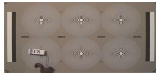
Figure 5, Zone Plate test chart
